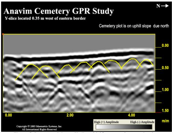
Figure 5: Interpreted data – Y-slice of 0.35 m west of eastern border.
