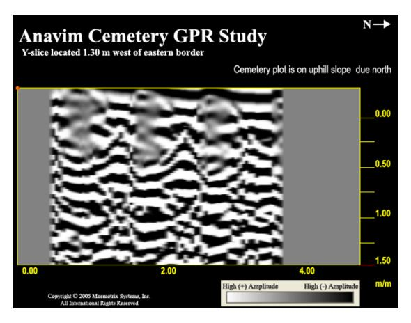
Figure 10: Raw data – 1.30 m west of eastern border. This Y-slice is located on the edge of the headstones, which can be seen here as three distinct "cloudy" areas. Note that because of the distinct change in material from concrete headstone to soil and sub-surface, it becomes difficult to "see" what lies below them. This area was markedly full of high positive amplitudes in the animation which was created for analysis in the original report.
