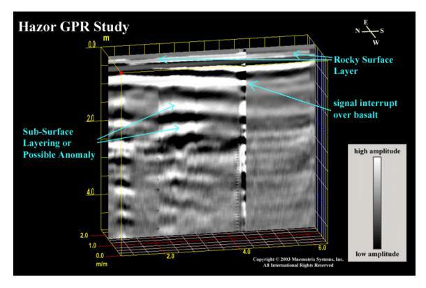
In a GPR study, high amplitude colors signify a strong reflection of the material, while low amplitude colors signify a weak reflection in the surrounding material or matrix. Therefore, when using the color table shown in Figure 3 above, where the contrast is strongest, there exists a strong difference between layers of sub-surface materials, which can be viewed as an anomaly or natural layering depending on the particular context.
